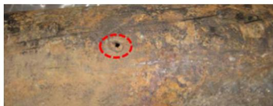
**Fig. 9** Through-wall defect. This pipe section was received from City West Water, Melbourne, Australia, for the investigation of carrying out research in RMIT, University, Australia. Internal corrosion of steel pipe. The fluid flowing through pipe causes stress corrosion. As a result, thickness of pipe is reduced from that particular area and a hole is developed
