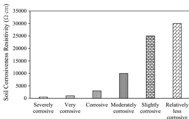
**Fig. 11** Corrosiveness of soil based on soil resistivity value. There is inverse relationship between soil corrosiveness and resistivity. As soil resistivity increases, corrosiveness decreases and vice versa
