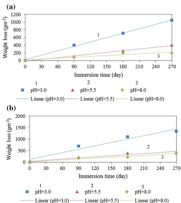
**Fig. 6** Comparison of corrosion in **a** steel and **b** cast iron under the influence of different pH value and exposure duration. At pH value of 3.0, the corrosion rate of cast iron was much higher than that of cast iron showing that steel is more resistive against the high acidic medium. However, for high pH values, steel and cast iron exhibited almost similar corrosion behaviour. Redrawn by the permission of the author Hou et al. (2016)
