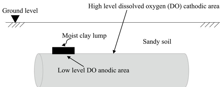
in soil include soil type, moisture content and degree of compaction. Figure 14 below illustrates the phenomenon of differential aeration. The disturbance in the soil layout can also yield different oxygen concentration; the undisturbed soil has less oxygen than disturbed soil due to its exposure to the open environment.
