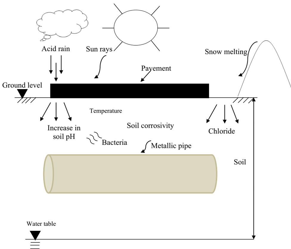
**Fig. 3** Mechanism of corrosion of metallic pipe in the soil. Chloride contents are added in soil through melting of glaciers in the summer season. Chloride retards the development of stable oxide layer on the metal surface which protects corrosion. Acid rain causes an increase
